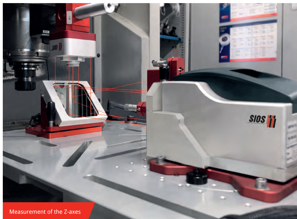
Compact measurement on a high-precision machine tool
